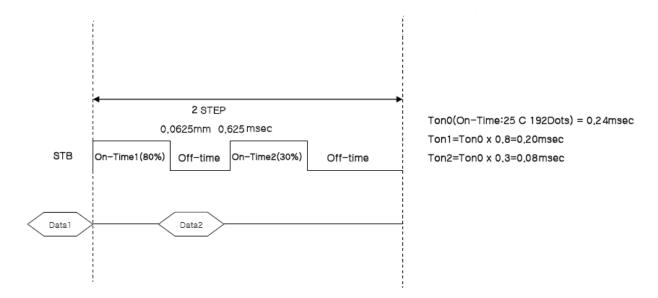
One dot will be printed by THP per two motor steps. The minimum off-time should be guaranteed since the heating element of TPH should be cooled down sufficiently in order to achieve good printing quality.
