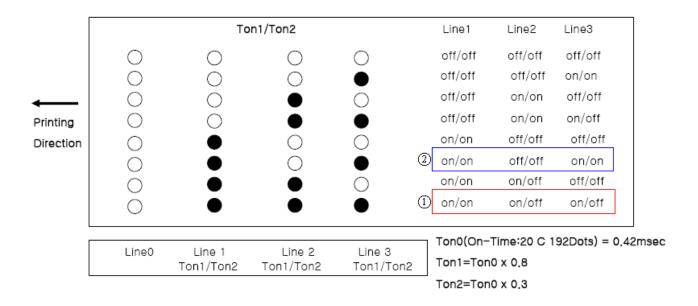
In case of the red box (4),both T-On 1 and T-On 2 should be in ON state since the previous dot was not printed in the Line 1, and only T-On 1 should be in ON state in case of Line2/Line3 since the previous dot was not printed in this case.
