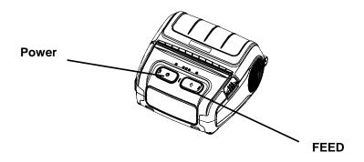
While the printer is turned off, turn on the printer while pressing the feed button. The printer setting values will then be printed.
