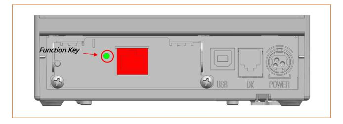
With the printer turned off, press the "Function Key" button and turn the printer on. After pressing and holding the "Function Key" button for about 5 seconds, release it. The factory reset occurs. Regardless of the current setting, DHCP mode is enabled.
