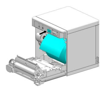
3) When you close the printer cover, the printer will enter the interface setting verification mode. For setting information, refer to the "Ethernet configuration" and "WLAN configuration" sections in SELF TEST INFORMATION.
