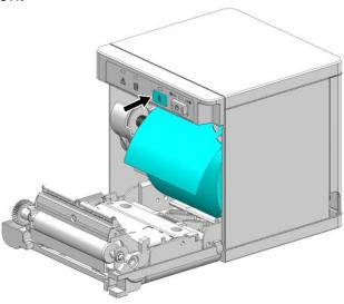
3) When you close the printer cover, the printer will enter the interface setting verification mode.
