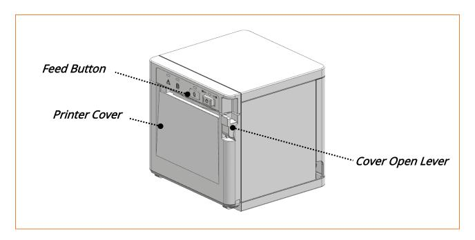
1) Open the printer cover after the printer has fully booted up.
