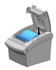
3) When you close the printer cover, the internal buzzer will beep 5 times and the printer will enter the interface setting verification mode. You will then see the following message printed out.
