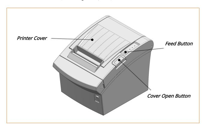
1) Open the printer cover after the printer has fully booted up.
