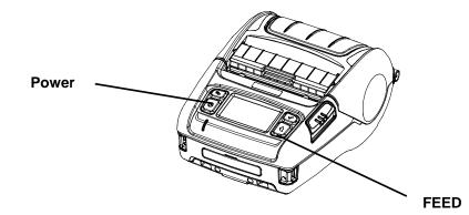
While the printer is turned off, turn on the printer while pressing the feed button. The printer setting values will then be printed. 3-1 Android Soft AP mode (default)
