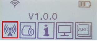
WLAN Factory reset is available in WLAN> ON / OFF> Factory Reset When the printer is turned off, the wireless LAN setting is applied as the factory default
